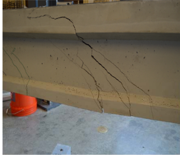
b) Shear cracks observed at ultimate load
