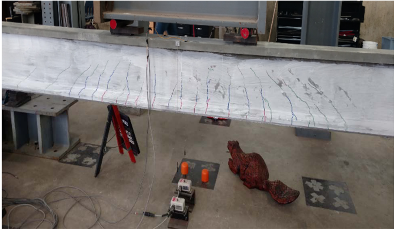
Figure 7: Crack Propagation at 37 kips
