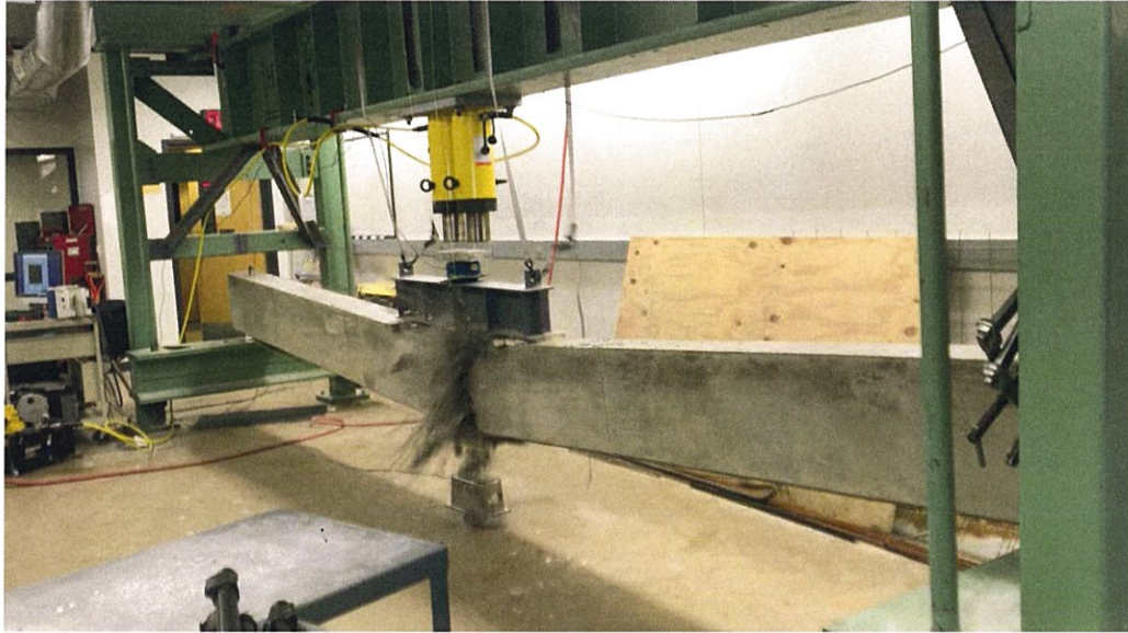
Figure A-7: Beam at Failure.
