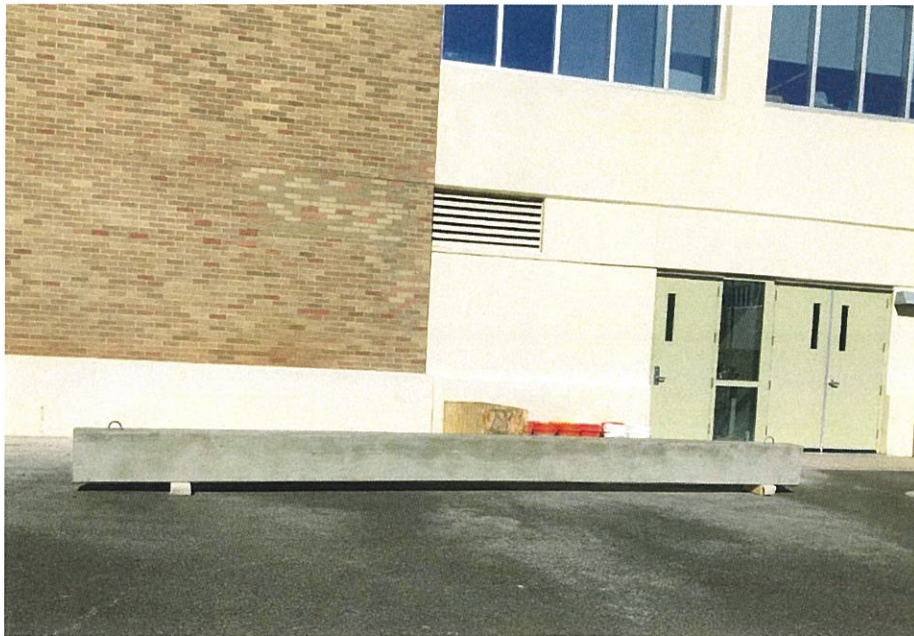
Figure A-6: Beam 28 days after Casting.
